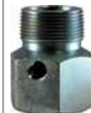
A2032 1 1/4" Relief Valve Adaptor Inlet: 1-1/4" MNPT Outlet: 1-1/4" FNPT Relief Outlet: 1/4" FNPT
