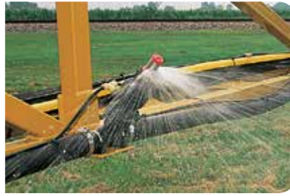
Nozzle can be mounted between 0° and 45°
